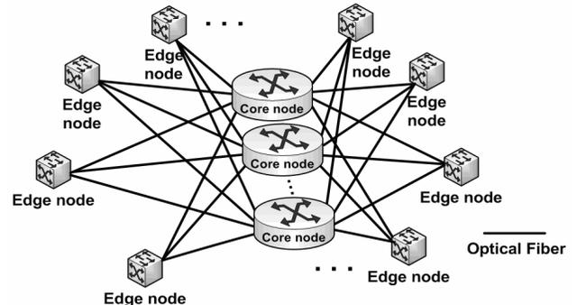
Fig. 2. Agile All-Photonic Network (AAPN) (OSN with several core nodes).
