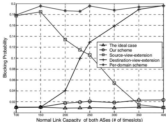
Fig. 8a: Overall network blocking probability of single path routing under varying normal link capacities.
