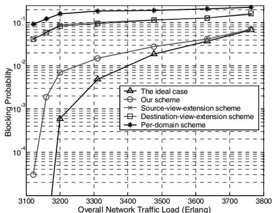
Fig. 8b: Overall network blocking probability of single path routing under various traffic loads with normal link capacity in both domains as 240 timeslots
