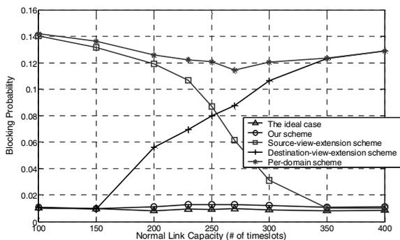
Fig. 9: Overall network blocking probability of diverse path routing under varying normal link capacities.
