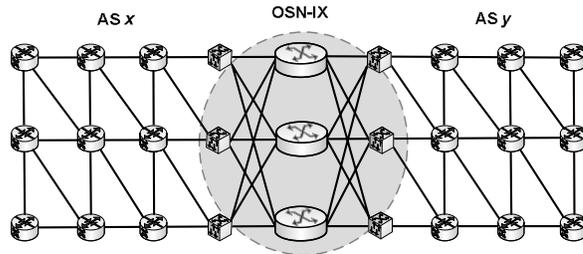
Fig. 7. Network topology used for simulation (27 nodes and 120 directional links in total) (we adopt AAPN as OSN).
