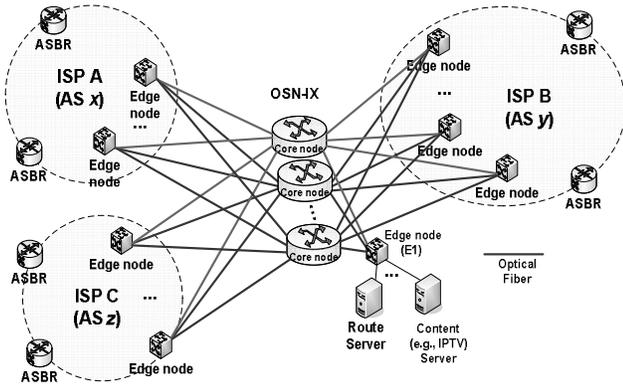
Fig. 3. OSN-IX implementation. There could be content servers (e.g., IPTV server) attached closely to core nodes to distribute contents efficiently).
