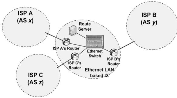
Fig. 1. A conceptual diagram of Ethernet LAN based IX [1,2,3].
