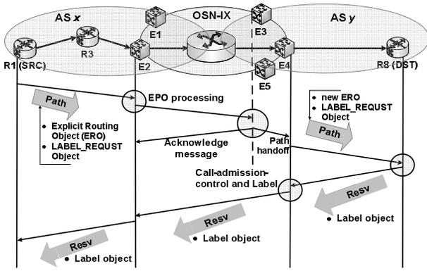
Fig. 5. Inter-ISP LSP signaling process that is fully based on RSVP-TE signaling protocol.
