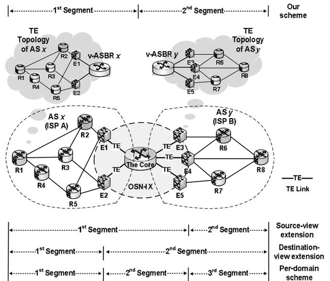
Fig. 4. OSN-IX's traffic engineering framework with example topologies of ISP A and ISP B, and three other inter-domain routing schemes (bottom).
